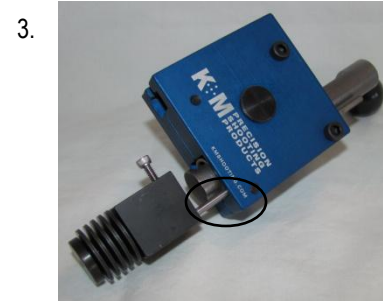
Remove press head from column and install force option on lower end of ram. Install force rod through clearance in upper left corner of head assembly as noted above.
