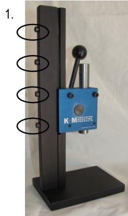
Loosen four column screws
